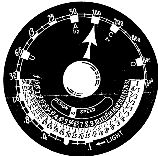
Weston Exposure Meter Control Dial Showing "A" and "C" Color Film Limits
