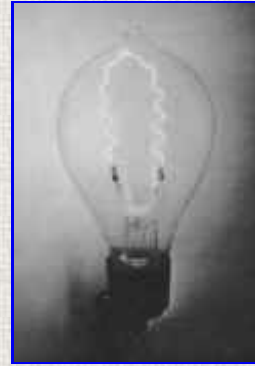
Weston incandescent light bulb with Tamidine filament
